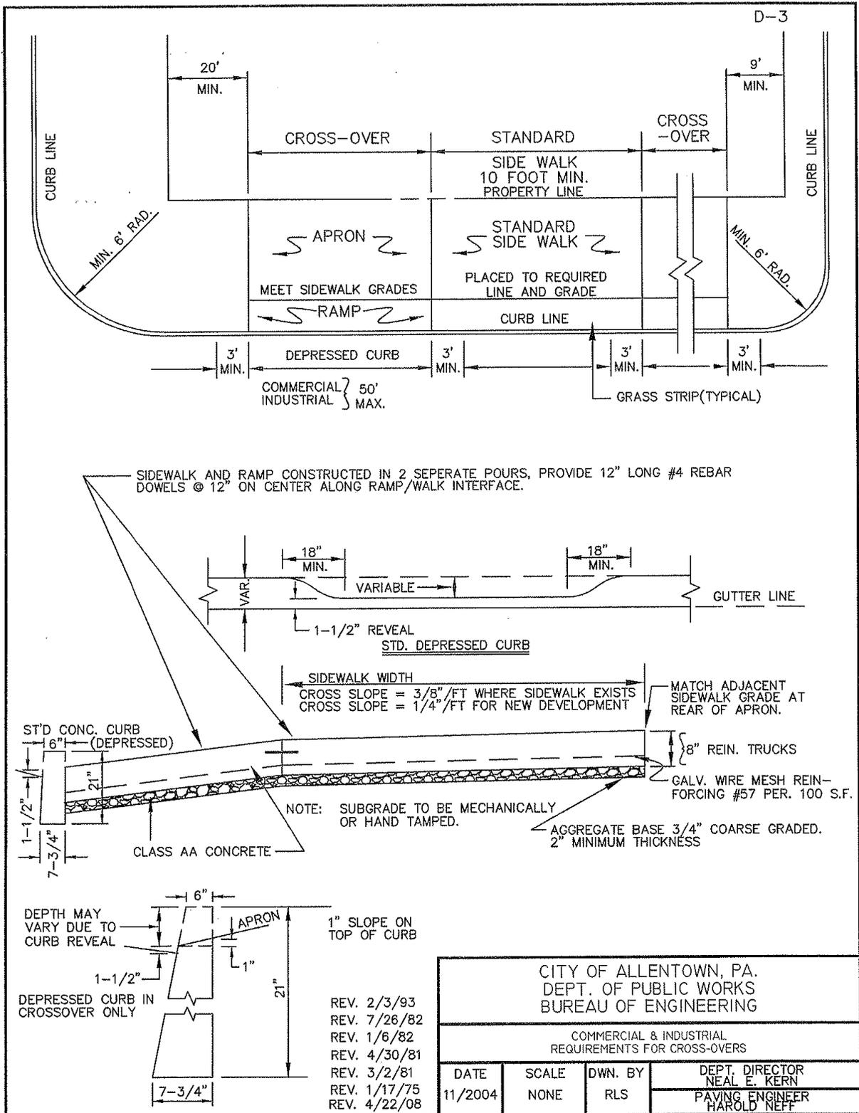
SIDEWALK AND RAMP CONSTRUCTED IN 2 SEPERATE POURS, PROVIDE 12" LONG #4 REBAR DOWELS @ 12" ON CENTER ALONG RAMP/WALK INTERFACE.
