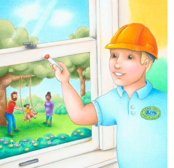
Using a test kit, the swab tip turns red. Now we know where there is lead.
